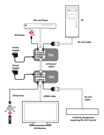
NOTE: The TX unit must have the female D-sub connector fitted, and the RX the male D-sub connector. There are no baud rate settings required as this is a pass through only
